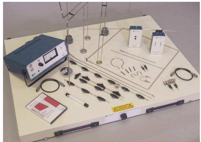
Ease of use of the equipment is further facilitated by a storage tray, which also serves as an inventory control for the various items (except the RF Generator) described below. This storage tray can be clipped on the ground plane for compact carrying purposes or can be fixed to a wall for easy access to the component parts.
