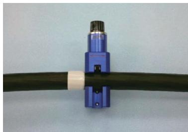
**STEP 3 :** Cut the cable laterally between the marked position.
